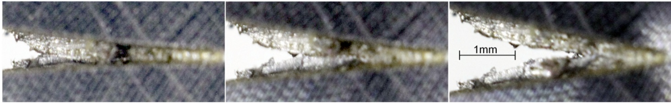
Fig. 14. Crack propagation behavior in the chevron-notched zone. The 12GBA tube steel in the UFG state.
